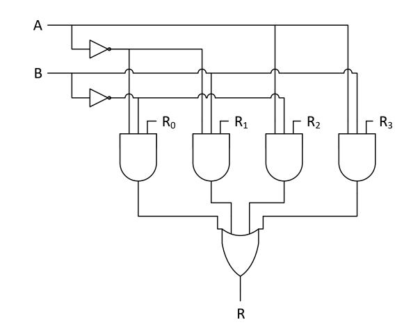
Sum-of-Products: With Specific Values for  $R_0$  through  $R_3$ , Terms are Removed and Simplified
